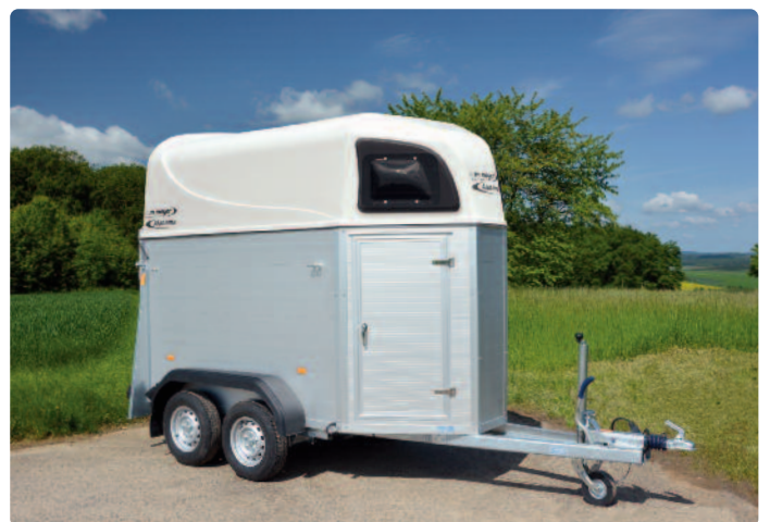
Alabama Alu Aluminiumwände, Servicetür, Polyesterhaube (weiß) Alabama Alu Panneaux en alu, porte de service, hardtop polyester (blanc) Alabama Alu Aluminium side panels, access door, polyester hardtop (white)
