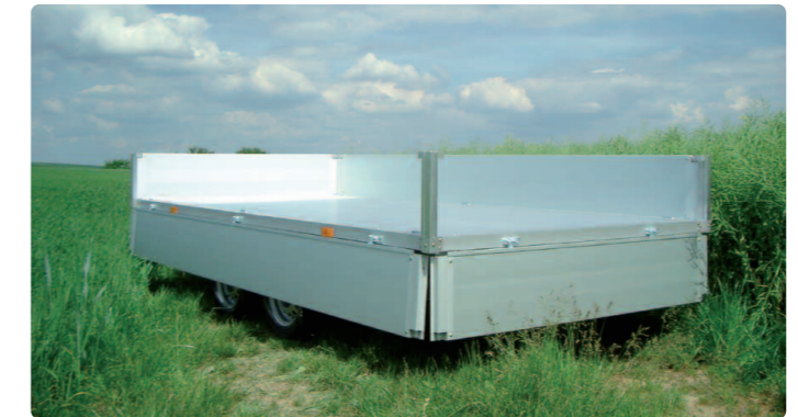
HLC 2746/186 Zubehör: Aluprofilboden HLC 2746/186 Options : plancher en aluminium HLC 2746/186 Optional extra: aluminium profile platform
