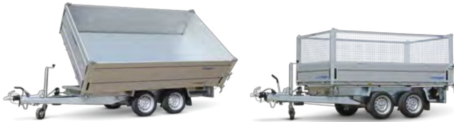
HKC 3031/186 Handpumpe, Zubehör: Alubordwanderhöhung HKC 3031/186 Pompe manuelle, option : ridelles supplémentaires en alu HKC 3031/186 Manual pump, option: additional aluminium side panels
