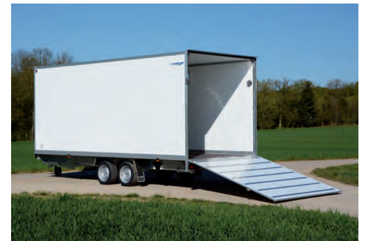
AZHLC 2750/210 Zubehör: u. a. Heckrampe (Traglast: ca. 700 kg) AZHLC 2750/210 Options : pont arrière (PTAC : 700 kg environ), etc. AZHLC 2750/210 Optional: ramp (carrying capacity: approx. 700 kg), etc.
