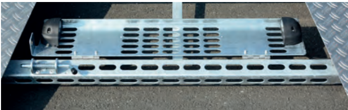
Nummernschildhalter (in Fahrposition und umgeklappt) Support de plaque minéralogique (position d'usage / de chargement) Number plate support (driving position / lowered to permit loading)
